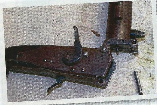
The gun opened up to show its firing mechanism.
